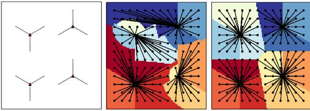
(a) Network topology (b) SINR as the Cost Function (c) Throughput as the Cost Function
